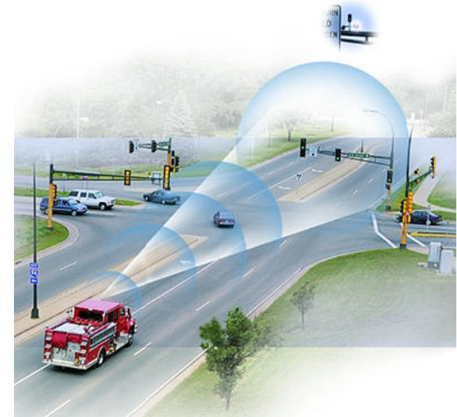
Traffic signal preemption
