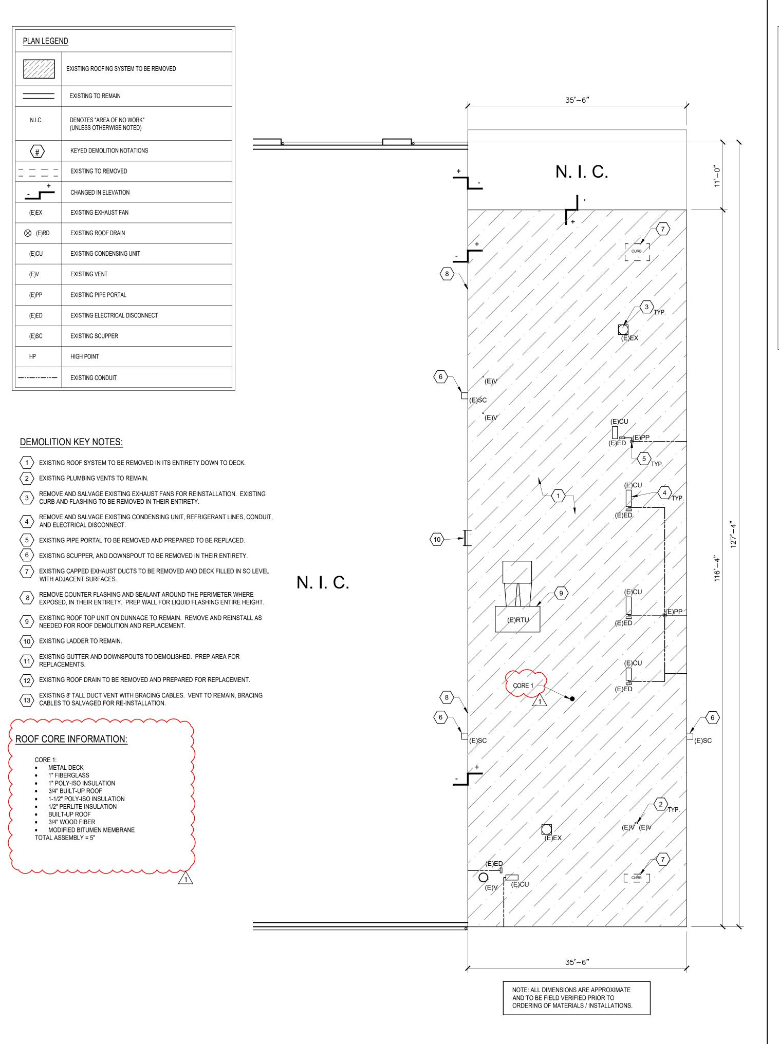
ROOF DEMOLITION PLAN
