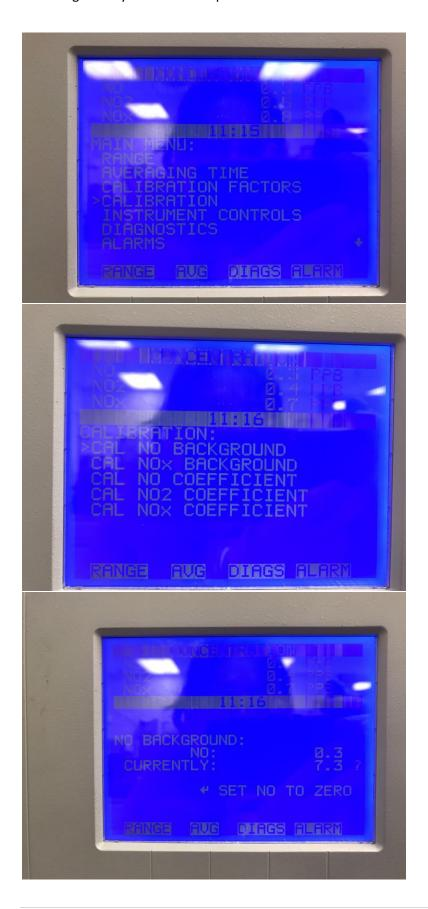
After the calibration sequence start 30 min, set the span 1. On the NOx gas analyzer, go to the main menu and choose 'Calibration'. Then choose 'CAL NO COEFFICIENT' and then calibrate NOx concentration and set the span concentration at 400 ppb. Also choose 'CAL NOx COEFFICIENT' and then calibrate the NOx.
